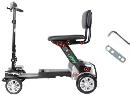
Photo 19. Check the screw loosening
