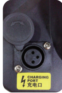
Photo 19. Then open the rear charging socket and insert the plug with a transfer connection
