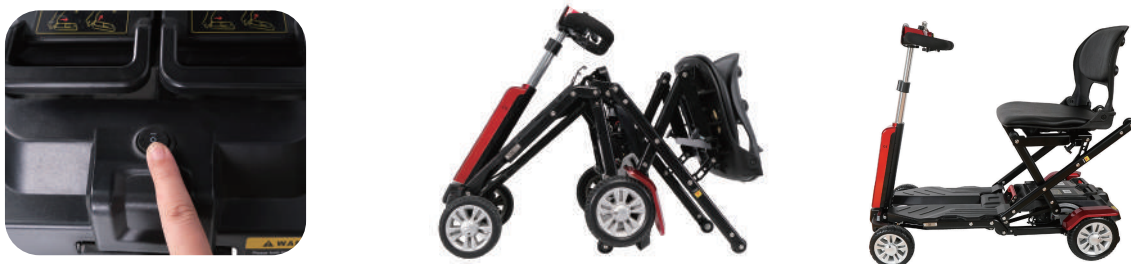
Photo 16. Electric switch unfold
