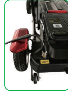
Photo 19. Then open the rear charging socket and insert the plug with a transfer connection
