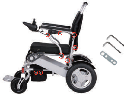
Photo 26. Check the screw loosening
