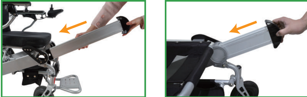
Photo 9. Installing the Battery
